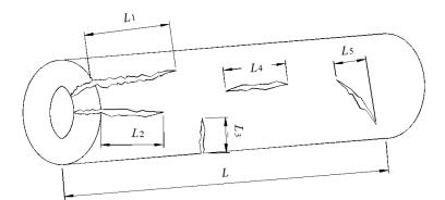
Fig. 3.5.2 Damage measurement (Cylindrical fender- Tear, Crack and Burn)
