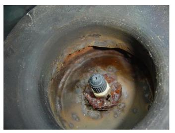
Photo 2.4.2 Separation of rubber body (Embedded plate)
