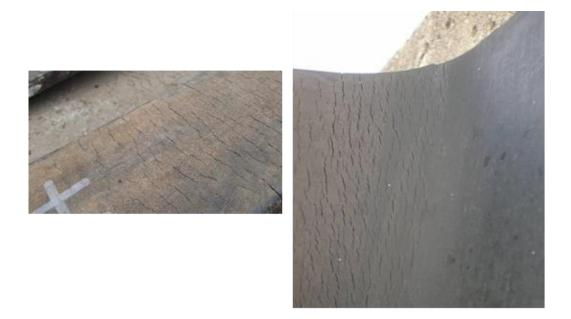
Photo 2.2.9 Ozone cracks on a rubber body
