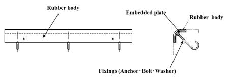
Fig. 2.6.2 Configuration of corner protector
