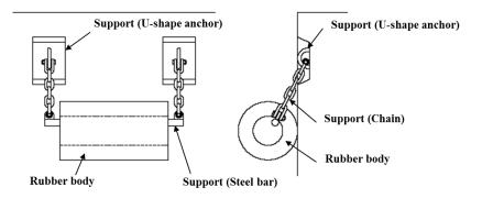
Fig. 2.5.1 Configuration of cylindrical rubber fender
