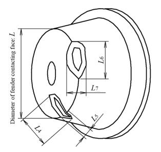
Fig. 3.2.8 Damage measurement (Drops, Missing rubber, Chipping and Wear - Circular fender)
