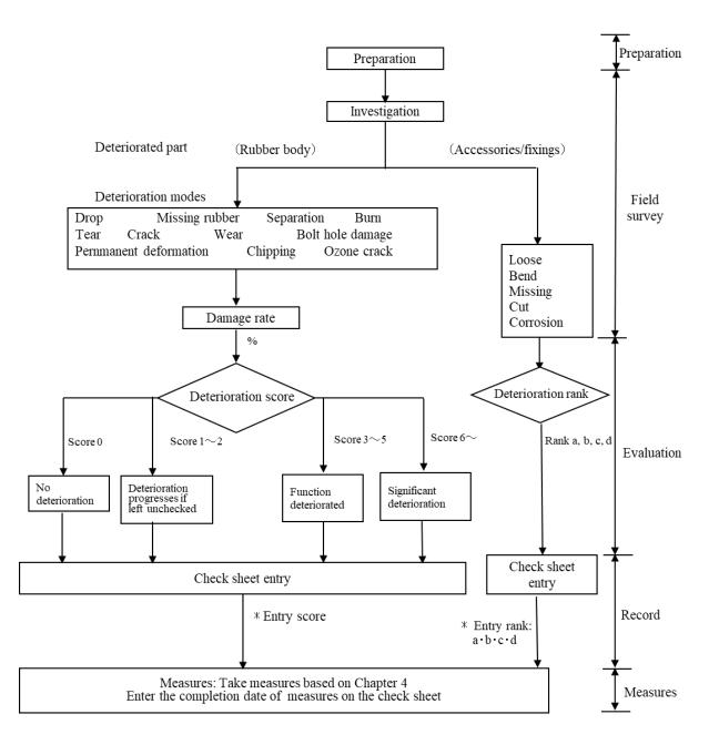
Fig. 3.2.1 Evaluation flow of check/diagnosis for V-type rubber fenders
