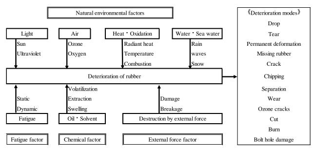
Fig. 2.1.1 Deterioration phenomenon and factors of rubber
