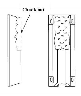
Photo 2.2.4 Missing rubber from rubber body
