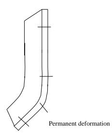
Photo C-3 Example of damage (Permanent deformation)
