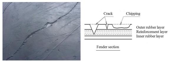
Photo 2.4.1 Cracking and chipping of rubber body
