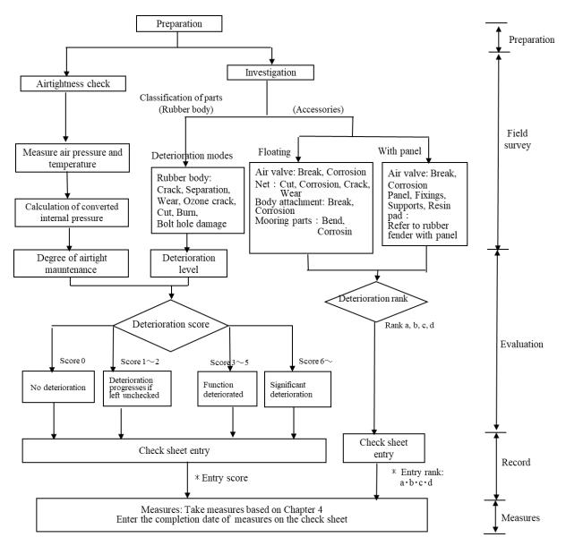
Fig. 3.4.1 Evaluation flow of check/diagnosis for pneumatic fender
