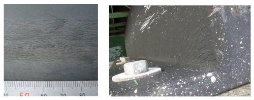
Photo 2.3.5 Ozone cracks on a rubber body
