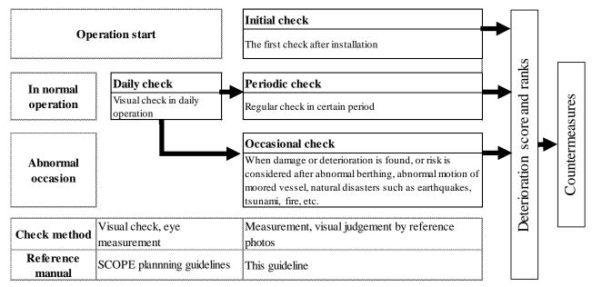
Fig. 1.4.1 Classification of checks and diagnoses
