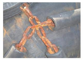
Photo 2.4.11 Corrosion of net
