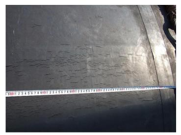
Photo 2.4.5 Ozone cracks on rubber body
