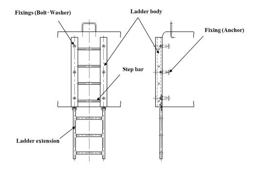
Fig. 2.6.1 Configuration of rubber ladder
