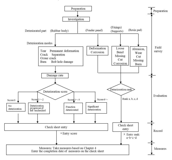
Fig. 3.3.1 Evaluation flow of check/diagnosis for rubber fender with fender panel
