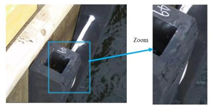
Photo 2.6.4 Missing rubber from rubber body
