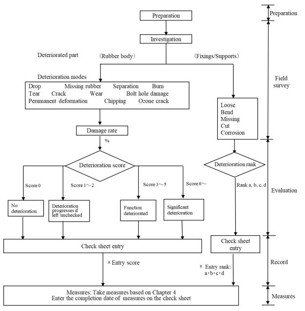
Fig. 3.6.1 Evaluation flow of check/diagnosis for other rubber equipment
