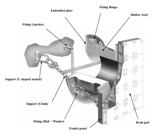
Fig. 2.3.2 Configuration of longitudinal rubber fender with panel
