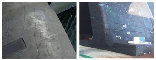
Photo 2.3.3 Crack in rubber body
