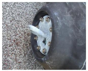
Photo 2.4.9 Malfunction of body attachment
