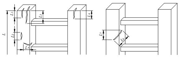
Fig. 3.6.2 Damage measurement (Crack - Rubber ladder)
