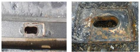
If the coated rubber is peeled off and the iron plate is exposed but there is no decrease in thickness, the failure rate is calculated as separation.
