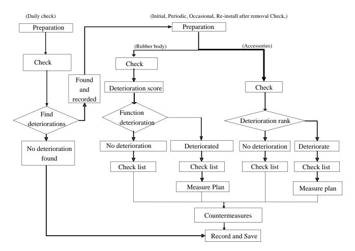
Fig. 1.3.1 The basic flow for implementing maintenance
