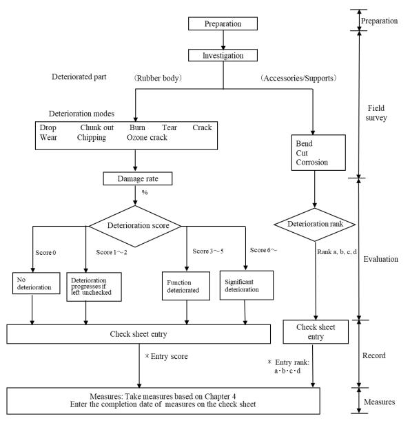
Fig. 3.5.1 Evaluation flow of check/diagnosis for cylindrical fender
