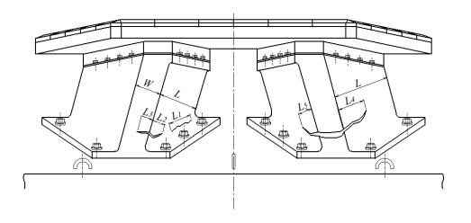
A leg B leg Note: These leg sides are expanded to show both sides Fig. 3.3.2 Damage measurement (longitudinal shape with panel)
