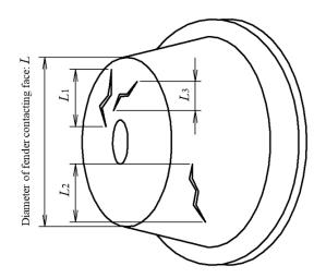
Fig. 3.2.7 Damage measurement (tears, permanent deformation, cracks, separation and burns - Circular fender)
