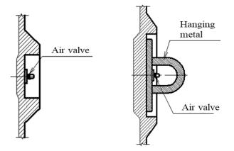
Fig. 2.4.3 Body attachment (floating type)
