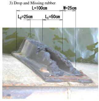
(Judge) Drop Missing rubber 50% 25 %  $\downarrow$   $\downarrow$  50% + 25 % = 75 % (Include in Drop) Total deterioration score 6 points
