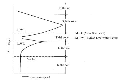
Fig. 2.1.2 Corrosion speed of steel in coastal area<sup>2</sup>)
