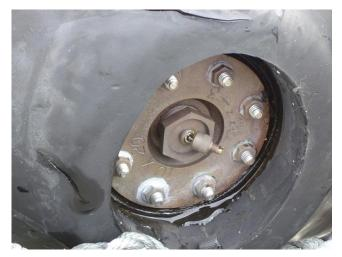
Photo 2.4.7 Malfunction of air inlet valve
