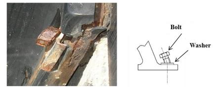
Photo 2.2.13 Bent fixing bolt (Accessories)
