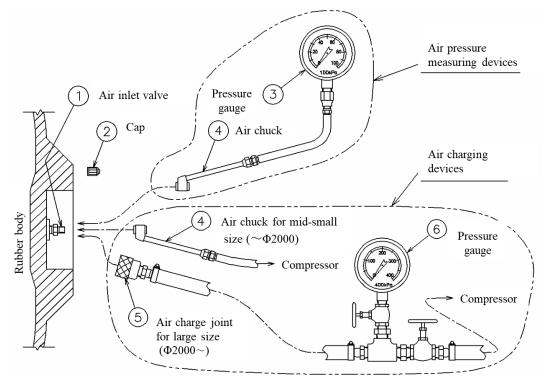
Fig. 3.4.2 Pressure measuring and air charge method (Floating type)
