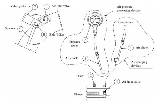
Fig. 3.4.3 Pressure measuring and air charge method (Fixed type with panel)
