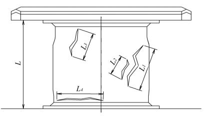
Fig. 3.3.3 Damage measurement (Circular shape with panel)
