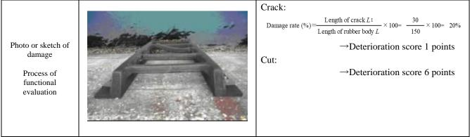
Fig. 3.6.6 Example of check sheet (Rubber ladder, Corner protector, Rubber net)
