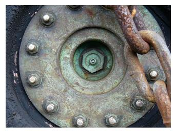
Photo 2.4.8 Corrosion of air inlet valve
