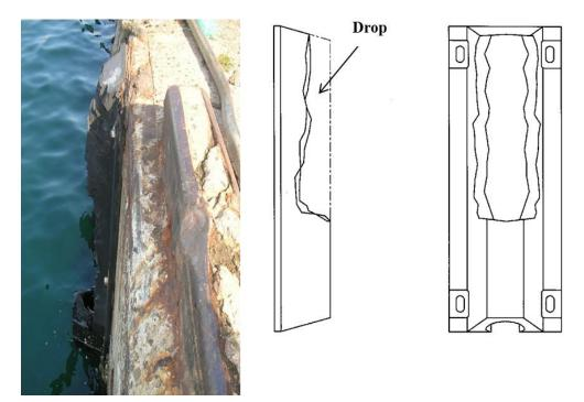
Photo 2.2.1 Drop of a rubber body
