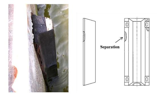
Photo 2.2.7 Separation of rubber body
