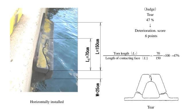
Photo C-2 Example of damage (Tear)
