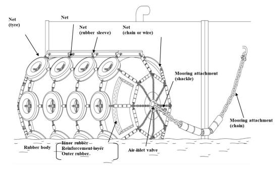
Fig. 2.4.1 Configuration of floating pneumatic fender
