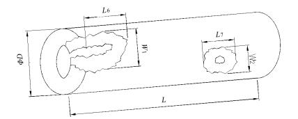
Fig. 3.5.3 Damage measurement (Cylindrical fender- Drop, Missing rubber, Chipping and Wear)
