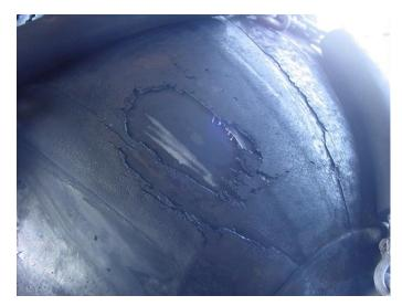
Photo 2.4.3 Separation of rubber body (Outer layer)
