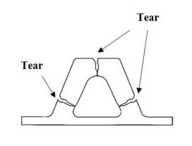
Photo 2.2.2 Tear of a rubber body
