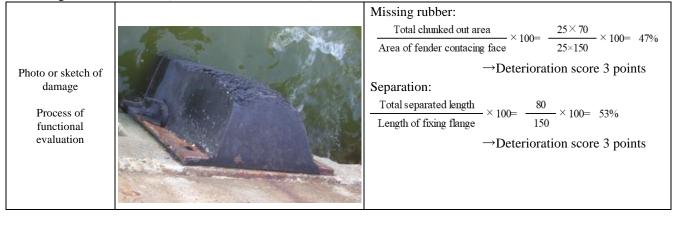
Fig. 3.2.9 Example of check sheet (V-type rubber fender)
