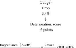
$\frac{\text{Dropped area } \{L_1 \times W\}}{\text{Area of contacting face } \{L \times W\}} =$  $\frac{25 \times 40}{25 \times 200} \times 100 = 20\%$
