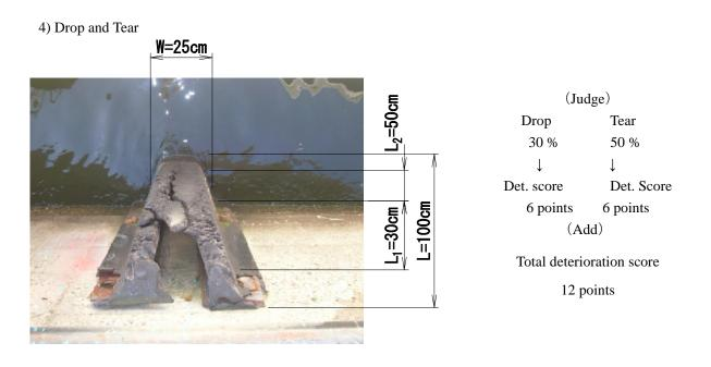
$$\frac{\text{Dropped area } \{L_1 \times W\}}{\text{Area of contacting face } \{L \times W\}} = \frac{25 \times 30}{25 \times 100} \times 100 = 30\%$$
