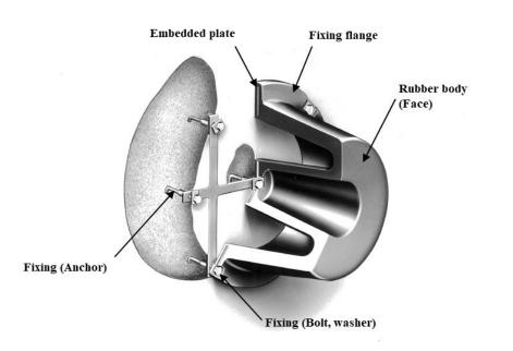
Fig. 2.2.2 Configuration of pivoted V-type rubber fender
