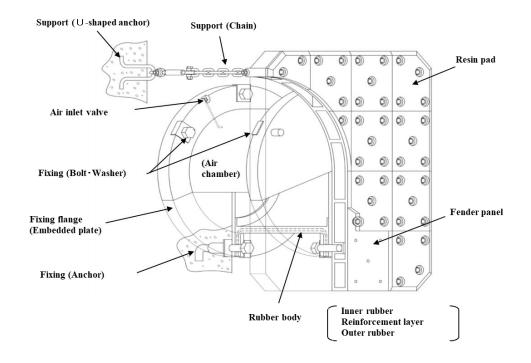
Fig. 2.4.2 Configuration of fixed-type pneumatic fender
