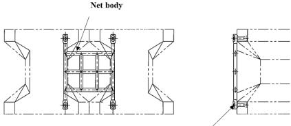
Fixings (Anchor · Bolt · Washer)
