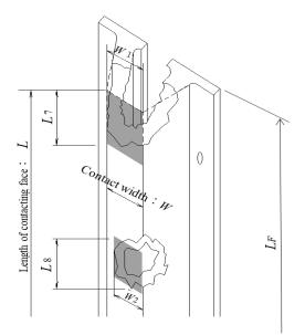
Fig. 3.2.4 Damage measurement (Drops, Missing rubber, Chipping, Wear)
