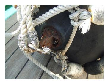
Photo 2.4.10 Corrosion of body attachment
