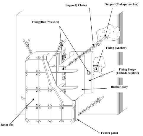
Fig. 2.3.1 Configuration of longitudinal rubber fender with panel
