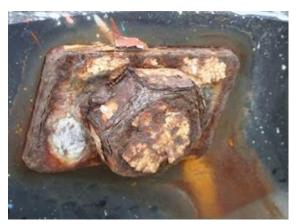
Photo 2.3.13 Corrosion of fixing bolt
