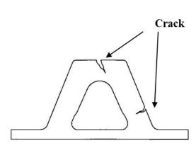
Photo 2.2.5 Cracks in rubber body
