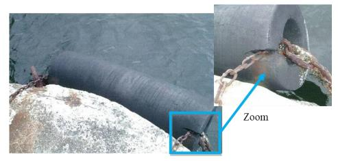
Photo 2.5.1 Crack of rubber body
