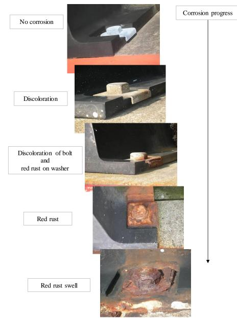
Photo 2.2.16 Corrosion of fixing bolt (Accessories)
