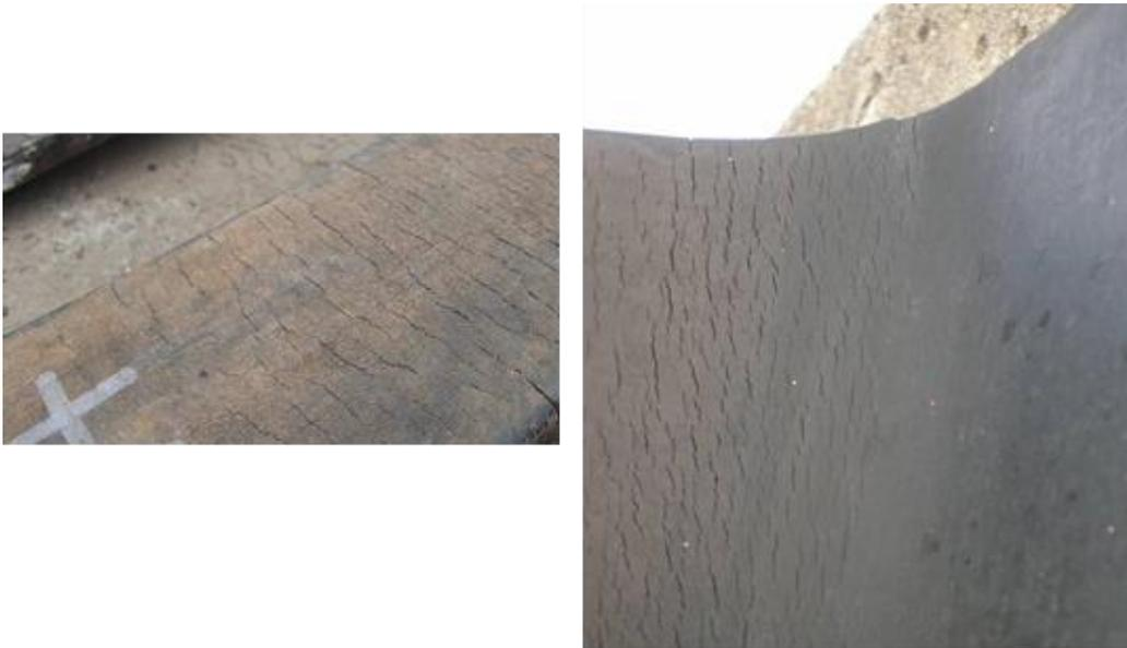
Photo 2.2.9 Ozone cracks on a rubber body
