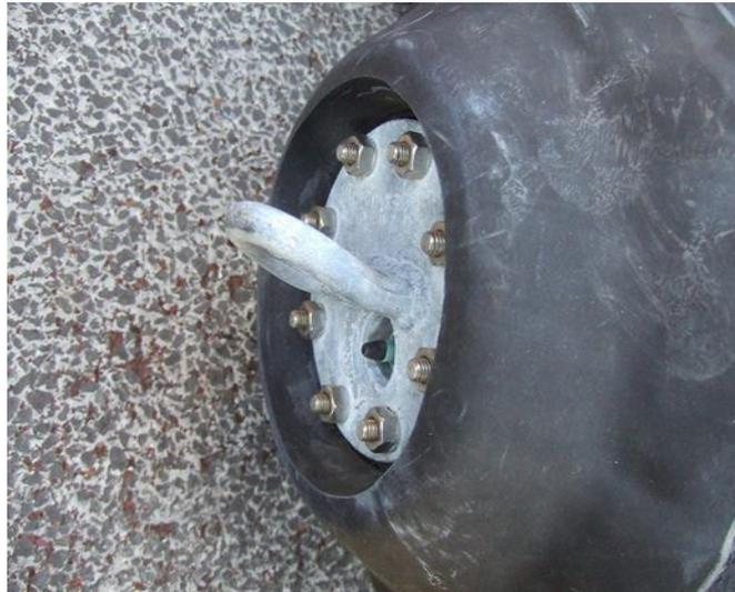
Photo 2.4.9 Malfunction of body attachment
