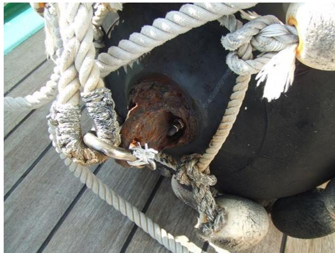
Photo 2.4.10 Corrosion of body attachment
