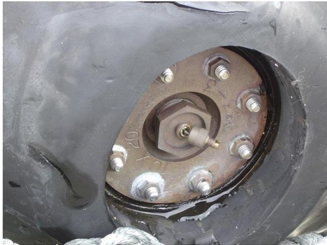
Photo 2.4.7 Malfunction of air inlet valve
