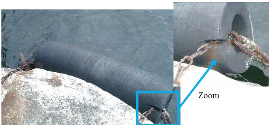
Photo 2.5.1 Crack of rubber body
