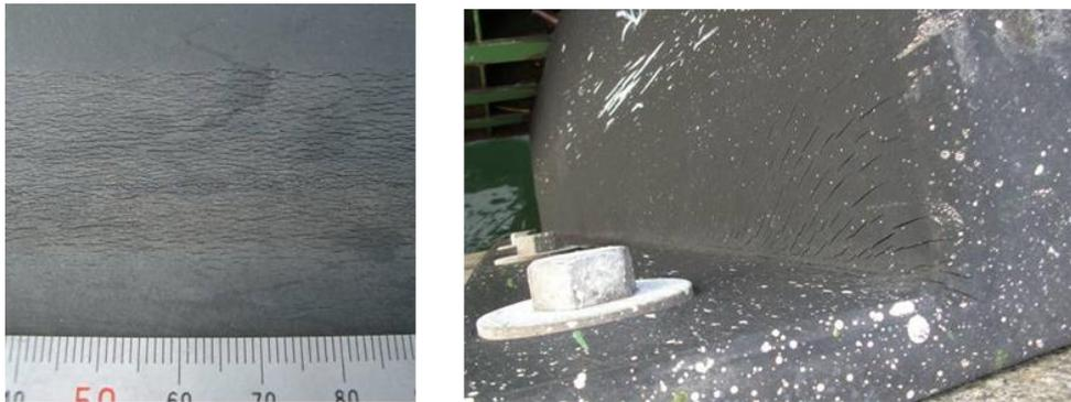
Photo 2.3.5 Ozone cracks on a rubber body
