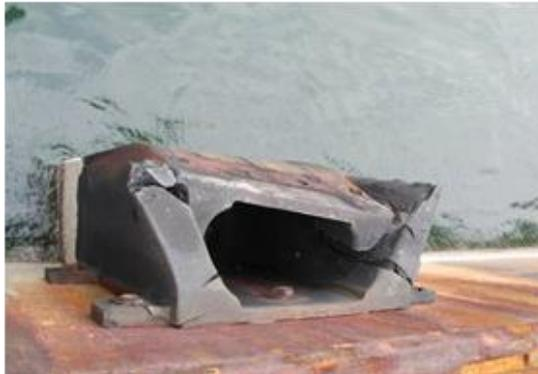
Photo 2.3.2 Permanent deformation of a rubber body
