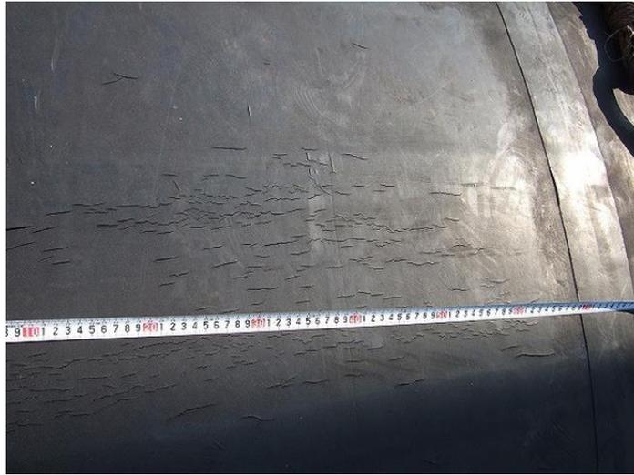
Photo 2.4.5 Ozone cracks on rubber body
