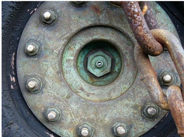
Photo 2.4.8 Corrosion of air inlet valve
