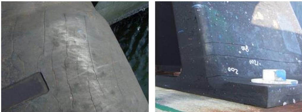
Photo 2.3.3 Crack in rubber body
