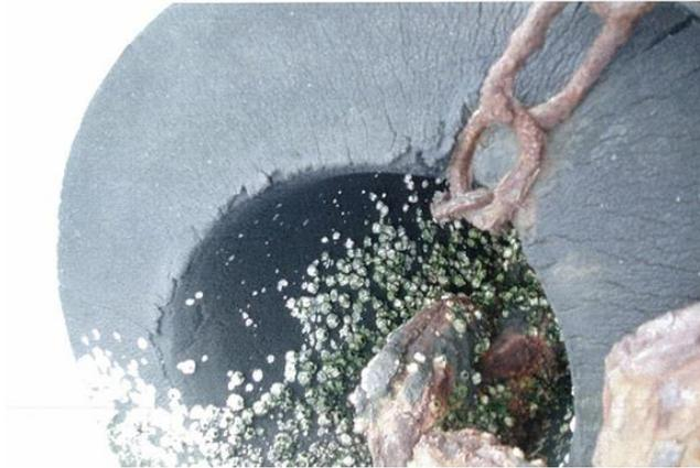
Photo 2.5.3 Ozone cracks in rubber body
