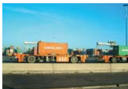
写真1 AGV (Automated Guided Vehicle)
