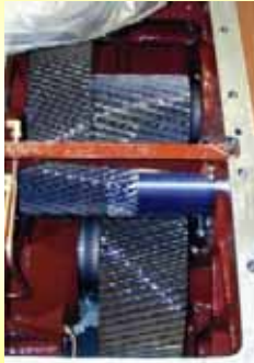
HS, IMS & MS Gear Teeth after Load Test
