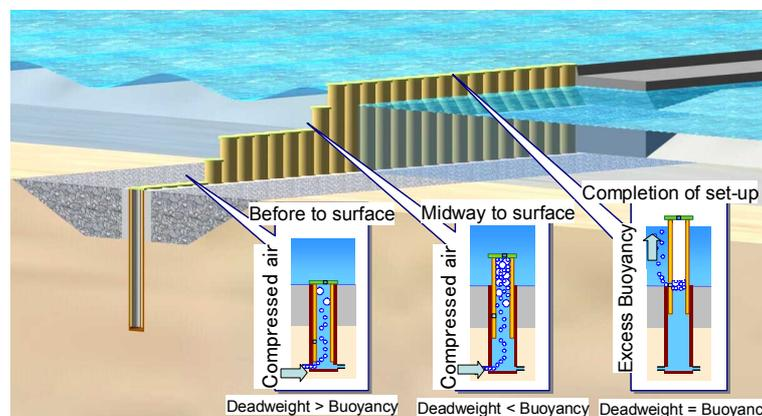
Figure 1 - Concept of the new breakwater
