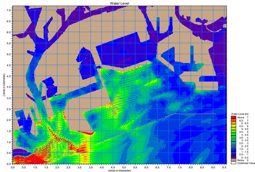
Figure 14. Tsunami Height Within the Ports of Los Angeles and Long Beach For A Hypothetical Event.
