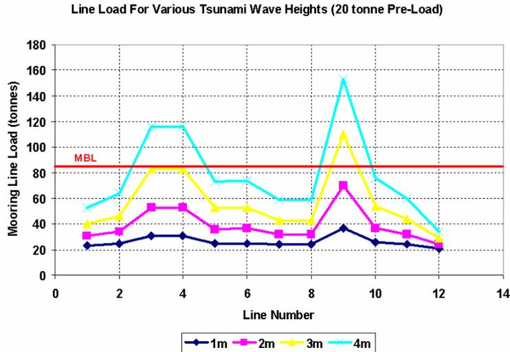
Figure 3. Mooring Line Analysis For Various Tsunami Heights (VWL).
