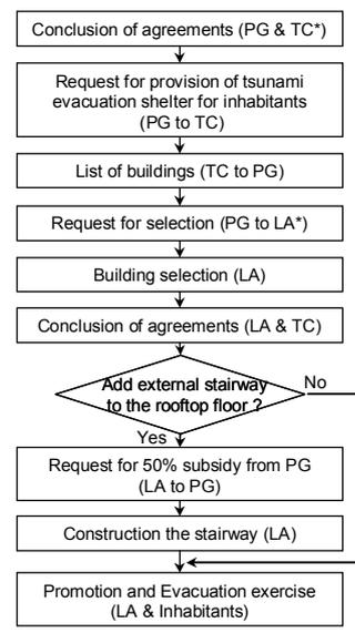
Figure 4: Flow diagram of utilization existing buildings as tsunami evacuation shelters
