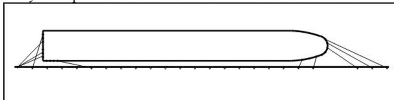
Figure 2. Typical Mooring line Arrangement for a Post-Panamax Container Ship.
