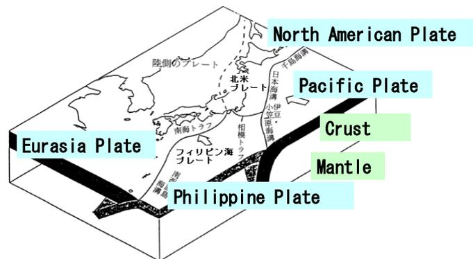
Fig. 1 Subduction zones and plates around Japan
