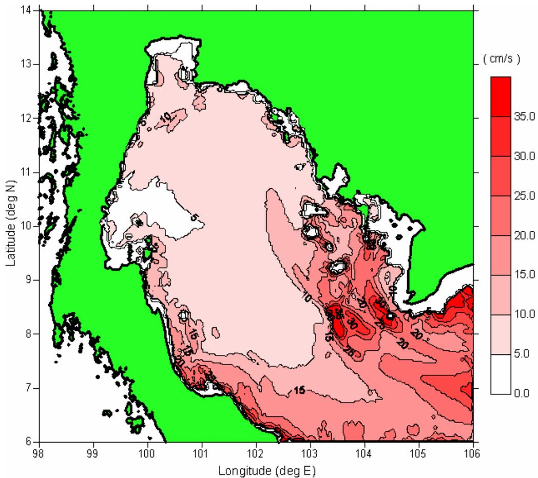
Figure 1: Current velocity from the Mw 9 earthquake
