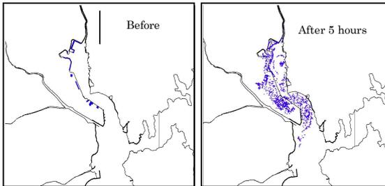
In Kesennuma Bay many of vehicles, vessels and aquacultural floats flow out in 5 hours after the earthquake as shown in Figure 2, while at Sendai port no container or timber out flow from the land side, except for some vehicles, due to the limited depth of inundation.
