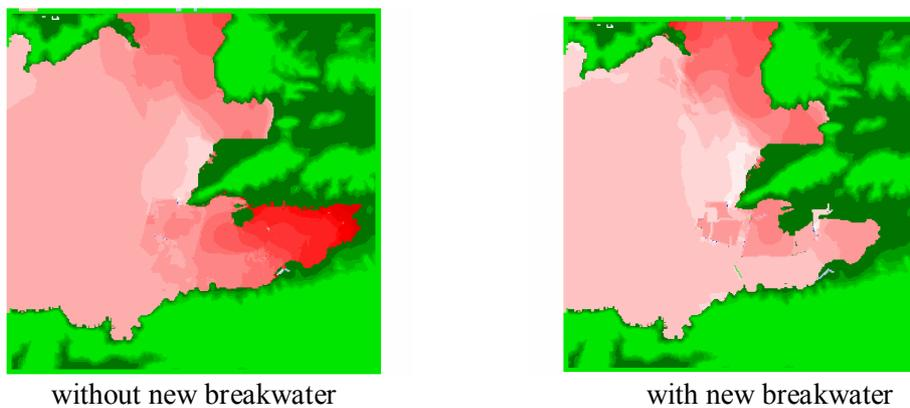
Figure 3 - Comparison of Tsunami height
