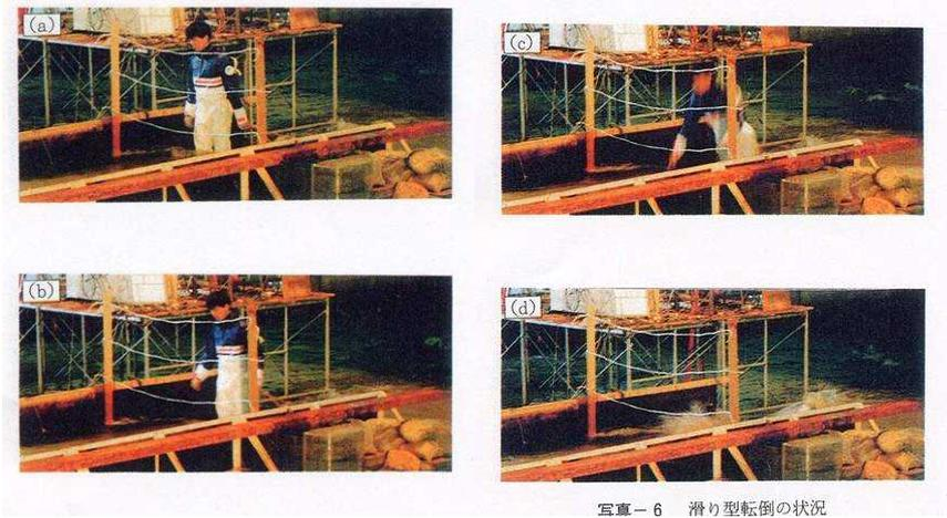
Figure 20 Stability tests of human bodies against currents
