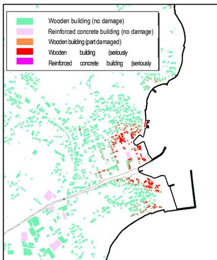
At Sendai port, buildings within the inundated area are all RC structures and the depth of water is limited. No destruction of buildings occurred.
