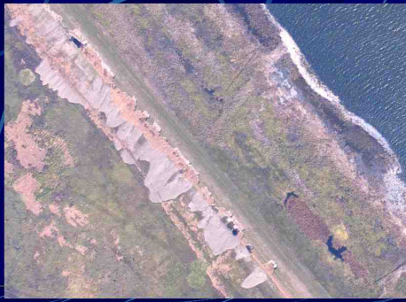
Overtopped Embankment - MRGO South Bank (Sand Core w/ sheetpile)
