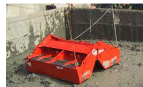
END construction method (which enables dredging thin layer and is environment-friendly)
