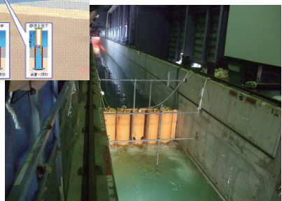
Experimentation of VTB in a long channel at Port and Airport Research Institute
