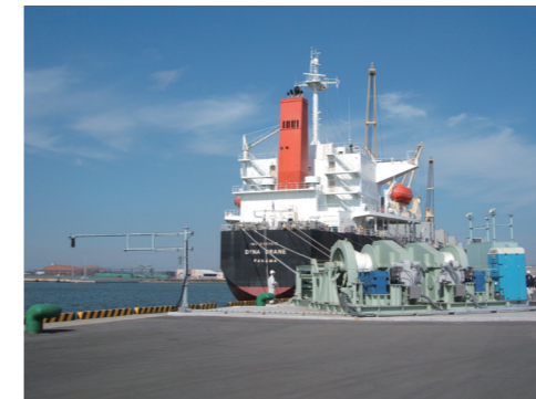
Vessel mooring system against long-period waves
